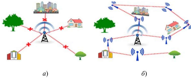
Fig. 1. (a) Obstructions are obstructing the mmWave signal. (b) Small cells are utilized to prevent multipath fading
